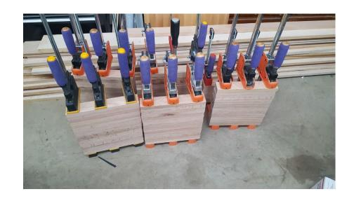
I use Elmers White Glue-All, interior. The boards are sitting on aluminum angle to elevate during glue application and clamping. The foam applicator can be placed in a zip lock bag and kept moist indefinitely.
