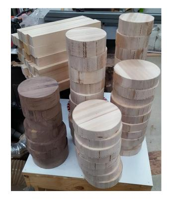
After removing from the clamps run the blocks through the thickness planner to make both sides smooth and parallel.
