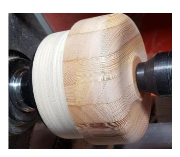
To hold the top while finishing the dome I use a Beall expanding collet. Other holding methods could be a jam chuck or vacuum.
