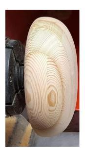
**Turn and sand the base.** The purpose of the concave feature would be to hold rings or a watch. I turn a slight concave on the base as well to insure the stand will sit flat. A few lines to decorate the base.
